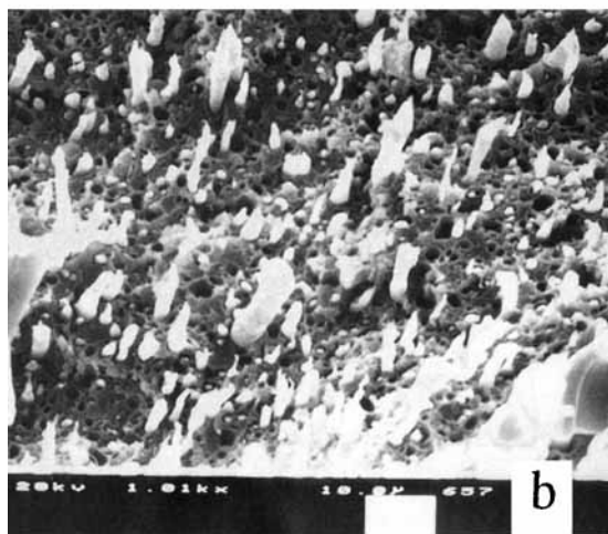
Figure 15 SEM micrographs of (a) skin and (b) core regions of injection molded MTBs of 75/25 PPO-PS/LCP blends.
